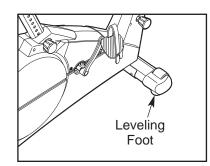
slightly during use, turn one or both of the leveling feet under the front stabilizer until the rocking motion is eliminated.
